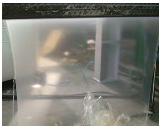
Figure 7. Modified PLA melt curtain. [Color figure can be viewed in the online issue, which is available at wileyonlinelibrary.com .]
